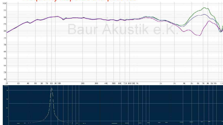
Frequency response measured on IAC baffle
